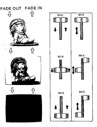
Fade-in and fade-out can be obtained by separately operating the Mix and Wipe Levers for EFFECT ③. If both fade levers are in the up position, move the left of them downward for picture to fade out. If this lever is subsequently moved top, the picture will fade in.
