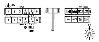
3) Select the vertical wipe mode on the Wipe Pattern Selector , and set the Mix and Wipe levers at middle position.
