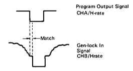
4) Adjust the H Phase Control for the Gen-lock ① to match the sync of both signals.
